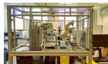
Assay plates are stored in a shaking incubator, and fluorescence or absorption is measured every 90 minutes using one of Eve's two microplate readers. Eve also has an automated microscope capable of taking both bright-field and fluorescence images across a broad range of wavelengths.
